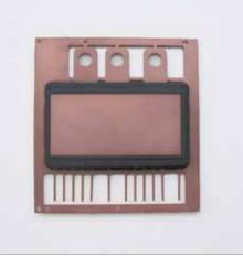
An integrated power module. These kind of customized modules, fully Ag-sintered, encapsulated and with double-sided cooling, are used for highly efficient inverters for EVs.
