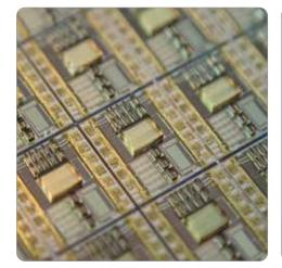
An optical multi-sensor wafer using Through Polymer Via (TPV) technology to create individual optical windows for each detector. This picture shows the wafer before singulation and assembly. Pictures above with courtesy of IC-Haus GmbH and Technical University of Delft.
