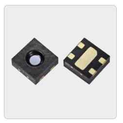
Humidity sensor on lead frame in QFN package. The top side shows an open (exposed) sensor area. The smallest window that can be designed with Film Assisted Molding is approximately Ø 0.30 mm.
