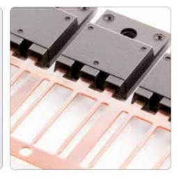
Power package in a TO-3pf/247 layout. This package layout is now also available with singleor double sided Ag-sintering (clip) for optimum thermal performance. " SMALLER, BETTER AND LOWER COST, WE REALIZE THE BEST PACKAGE FOR YOUR PRODUCT "
