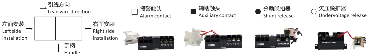
脱扣器安装方式及附件代号 Release installation method and accessory code
